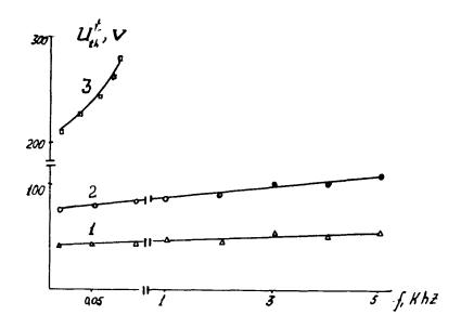
FIGURE 2. The frequency dependences of the threshold voltages, which occured in planar (1,2) and homeotropic (3) texture smectic A phase  $1.3 - 0 = 2.10^{-9}$ ,  $2 - 6 = 10^{-9}$  ohm<sup>-1</sup>. cm<sup>-1</sup>;  $t = 25^{\circ}$ C.
