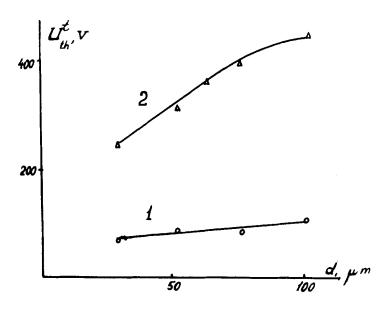
FIGURE 3. The dependence of threshold voltage instability, occurring from planar (1) and homeotropic (2) texture on the electrooptical cell thickness.
